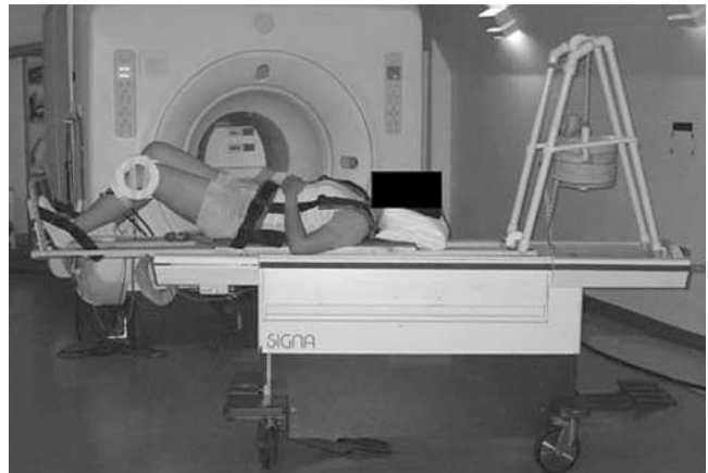
Figure 1. Photograph shows the subject set up on the nonferromagnetic loading device used for imaging. This device allowed the subjects to do unilateral knee extension in the supine position. Resistance to knee extension was accomplished by pushing against a footplate that was connected (through a pulley system) to a moveable carriage containing epoxy weights. (Reprinted with permission from Salsich GB, et al: In vivo assessment of patellofemoral joint contact area in pain-free individuals. Clin Orthop , in press.)
